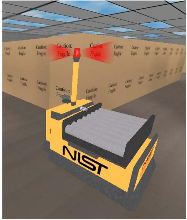
Figure 2: A performance metric that tests required AGV side clearance during turns and its virtual representation. This metric provides an adjustable width passageway. The robot is repeatedly driven through the metric with the width of the metric being reduced after each run.
