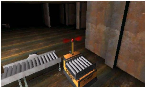
Figure 3: Example of a Unit Loader AGV approaching a loading station for docking.
